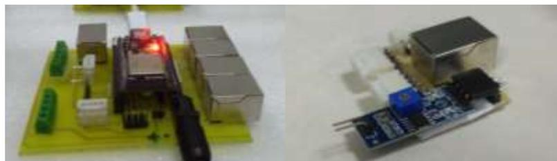
Gambar 3. board hardware nodemcu esp 32s dan connector sensors
