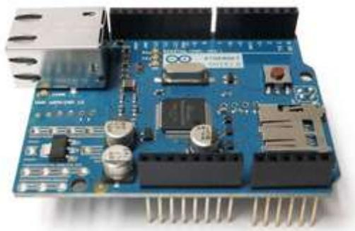
Gambar 5. Ethernet Shield
